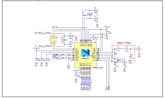
Figure 3. Traditional discrete solution for nRF24LE1
