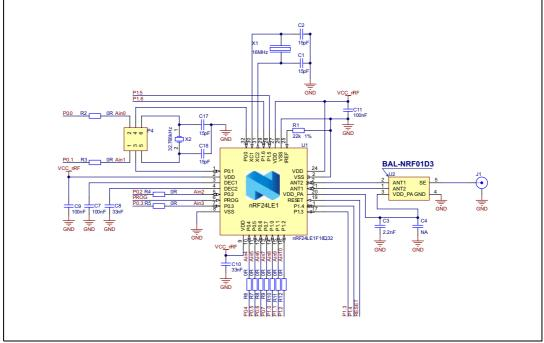
Using BAL-NRF01D3 **no external components** are required for matching and for harmonic filtering. Only a 2.2 nF external capacitor is required for  $V_{DD}$  decoupling. The test board for nRF24LE1 is shown in *Figure 8*.
