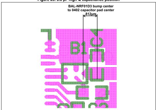
Figure 23. 0.8 pF high Q capacitance position
