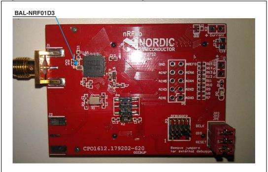
Figure 14. nRF2752 ST balun reference nRFgo module from Nordic Semiconductor
