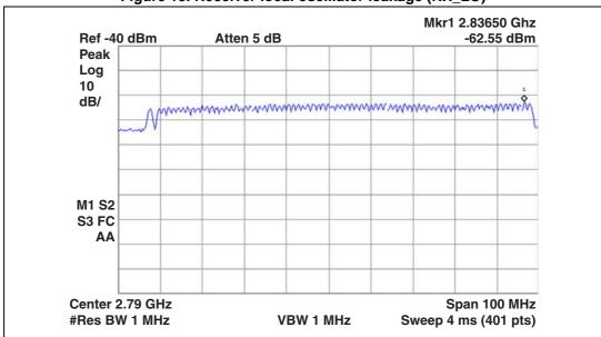
Figure 13. Receiver local oscillator leakage (RX\_LO)
