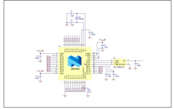
Using BAL-NRF01D3 only a 0.8 pF capacitor is needed for molding and for harmonic filtering. A 2.2 nF external capacitor is required for  $V_{DD}$  decoupling. The test board for nRF51822 is shown in *Figure 14*.
