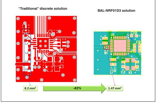
Compared to discrete solutions, the BAL-NRF01D3 solution is much easier to implement.
