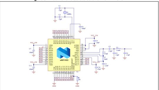
Figure 5. Traditional discrete solution for nRF51822
